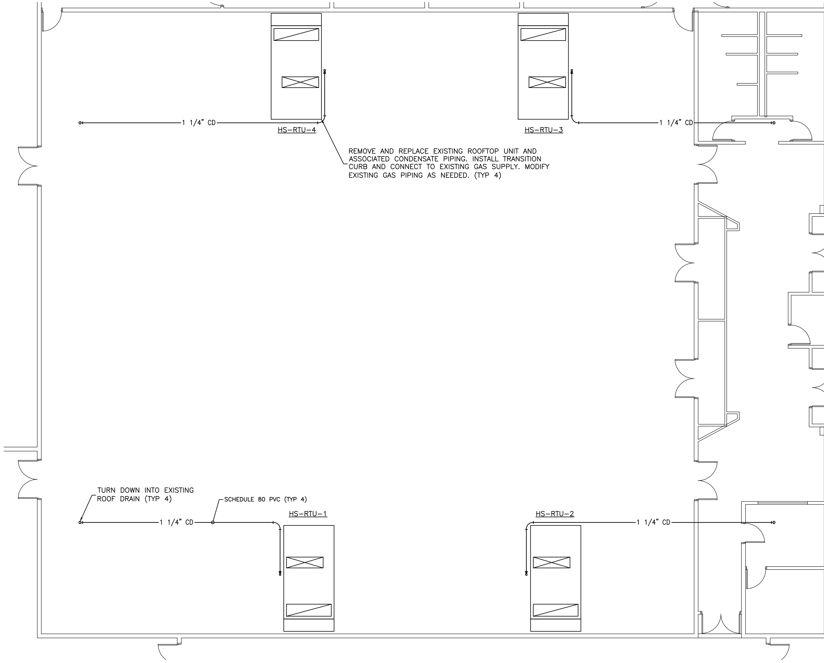
3 HIGH SCHOOL MECHANICAL HVAC PLAN - GYM SCALE: 1/8"=1'-0"
